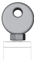
Installation correcte PATROLMED sur le support TOWER - TOWER22 - TOWERA2
